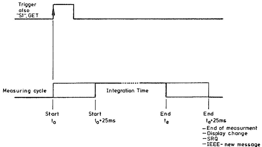
Range and function switching operations carried out shortly before triggering may lead to delay times of up to 225 ms.
