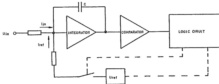
fig.1 Simplified block diagramm
