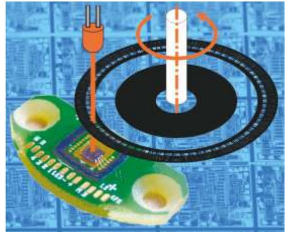
Resolutions of up to 5000 increments at 40 mm track diameter have been realised. PREMA uses an innovative, patented method to form sharp index pulses.
