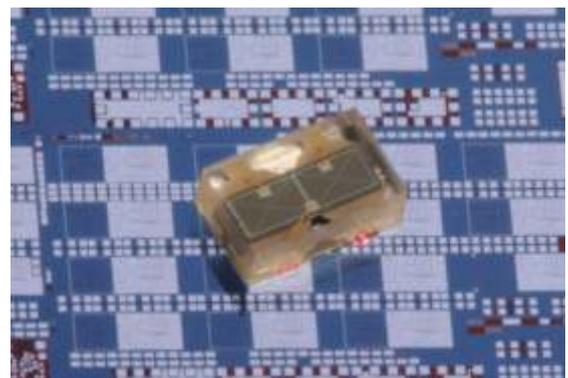
variable gain amplifier, bandpass filter, integrator and digital output stage. This configuration allows a very easy assembly in a tiny package. Filter and adaptive gain control give it an unmatched rejection of disturbing signals.
