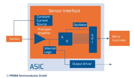
The sensor is supplied with a constant current from the sensor interface. The ASIC additionally includes a sensor signal amplifier and an A/D converter, which transmits its output over the integrated SPI interface to an external microcontroller.
